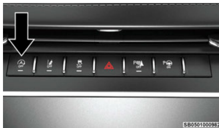
Stop/Start OFF Switch
