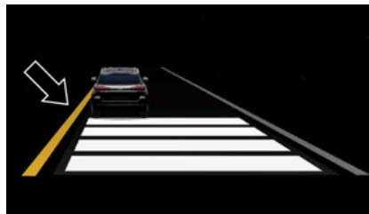
Lane Crossed (Flashing Yellow Line)
