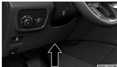
Interior PDC Location
