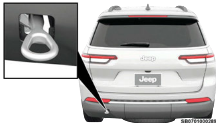
Rear Tow Hook Installed
