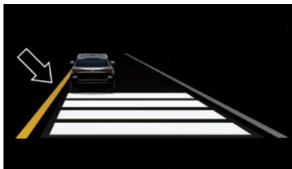
Lane Crossed (Flashing Yellow Line)
