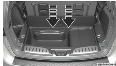
Pulling Down The Carpet Floor Panel To Access Top Tether Strap (3rd Row Bench)
