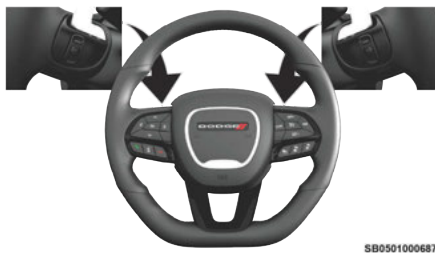
Remote Sound System Controls
