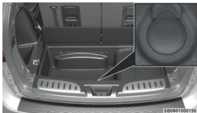
Winch Plug Location
