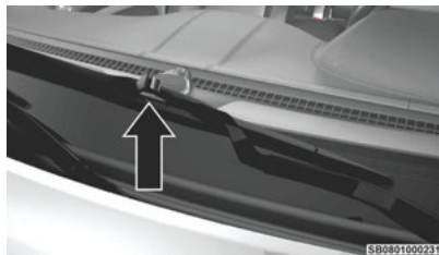
Wiper Blade With Release Tab In Unlocked Position
