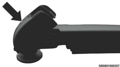
Wiper Pivot Cap In Unlocked Position
