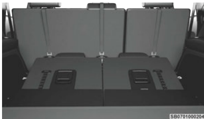
Second Row Bench Seat Top Tether Strap Mounting (7 Passenger Seating)
