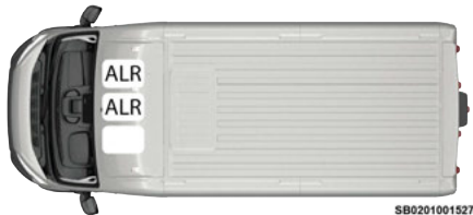
Front Bench Seat: Switchable Automatic Locking Retractor (ALR) Locations - Gas Models
