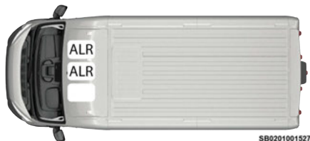
Front Bench Seat Automatic Locking Retractor (ALR) Locations (Gas Models) — If Equipped
