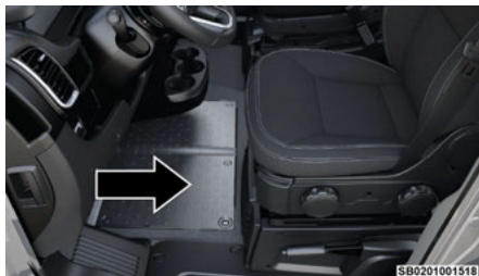
Battery Access Panel
