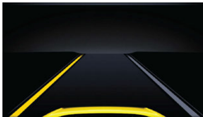
Lane Approached (Flashing Yellow Lane Line) With Yellow Telltale
