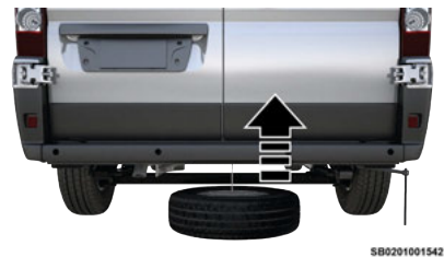
Damaged Wheel Stowage
