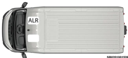
Front Bucket Seat: Switchable Automatic Locking Retractor (ALR) Location - Gas Models
