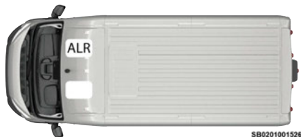
Front Bucket Seat Automatic Locking Retractor (ALR) Location (Gas Models) — If Equipped
