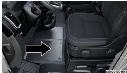
Battery Access Panel
