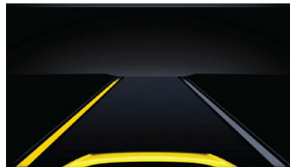
Lane Sensed (Solid Yellow Lane Line) With Solid Yellow Telltale
