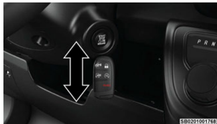
Depleted Key Fob Battery Procedure
