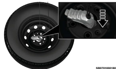
Reinstalling The Retainer
