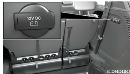
Rear Power Outlet
