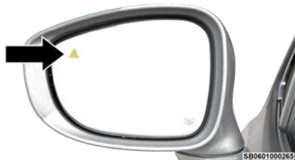
Warning Light Location
