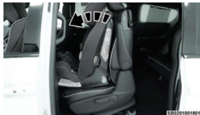
Easy Tilt With Child Seat Installed
