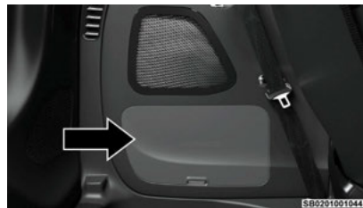
Vacuum System Access Panel
