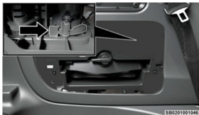
Vacuum Hose Release Lever
