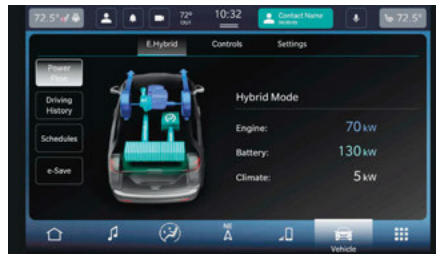
Power Flow Screen
