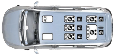
Eight Passenger Automatic Locking Retractor (ALR) Locations
