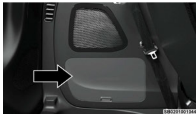
Vacuum System Access Panel
