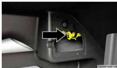
Fuel Door Emergency Release
