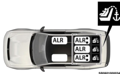
ALR — Switchable Automatic Locking Retractor
