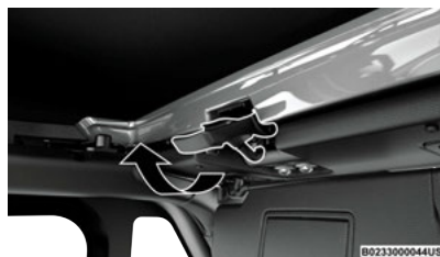
Engage Both Header Latches
