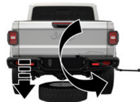
Pulling The Spare Tire Out
