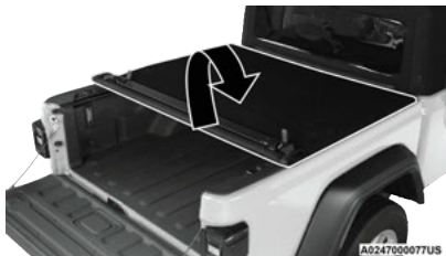
Roll Tonneau Cover Forward
