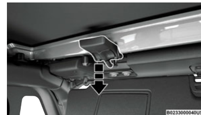
Release Both Header Latches
