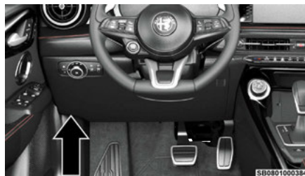
Interior Fuse Box Location
