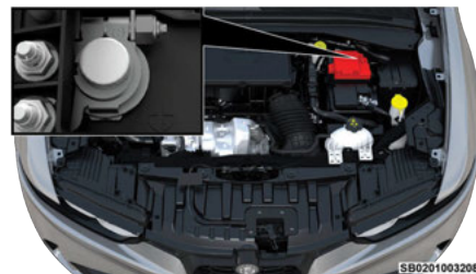
Positive (+) Battery Post
