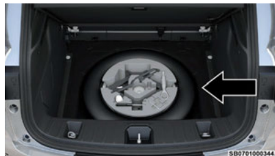
Damaged Tire Stowage
