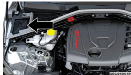
Under Hood Fuse Panel Cover
