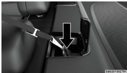
Upper Tether Anchorage Location
