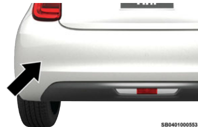
Ultrasonic Sensors Location
