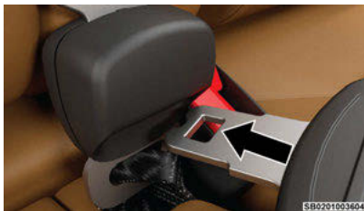
Disengaging The Latch Plate From The Buckle
