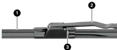
Wiper Blade With Release Tab In Locked Position
