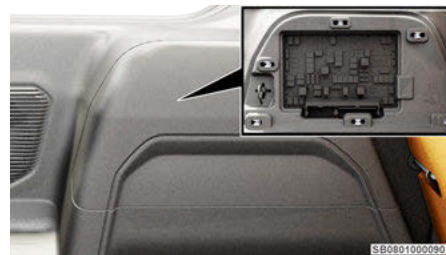
Rear Power Distribution Center Location
