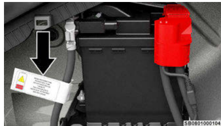
Negative Battery Cable Label Location
