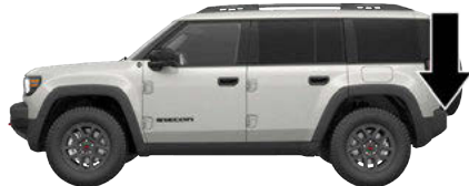
BSM Radar Location (Left Side Shown)
