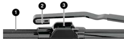
Wiper Blade With Release Tab In Unlocked Position
