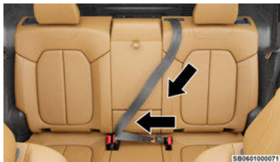
Inserting Latch Plate Into Buckle
