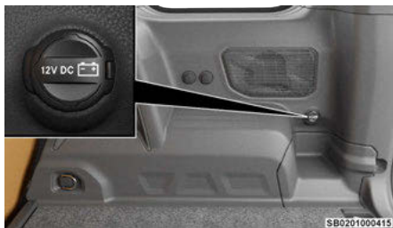
Rear Power Outlet
