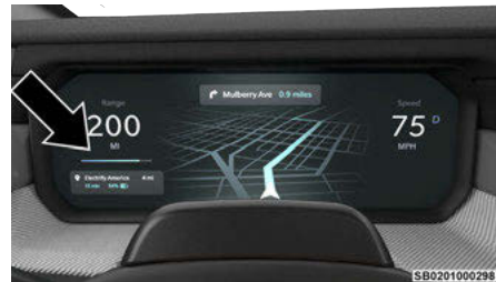
High Voltage Battery Display
