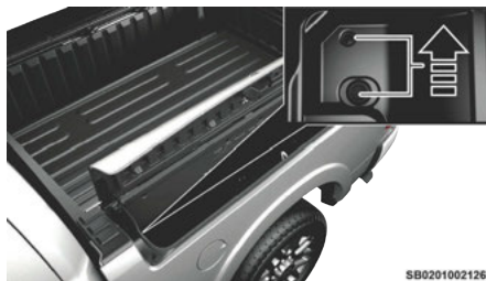
RamBox Drain Plug Removal
