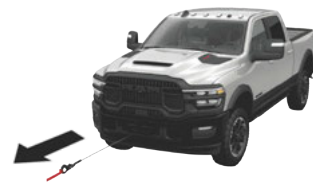
Pulling Synthetic Rope Under Tension
