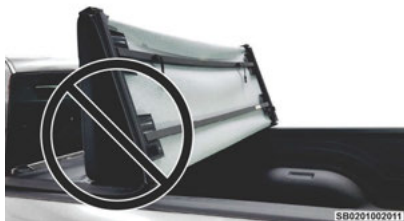
Incorrect Folding — Will Cause Damage
