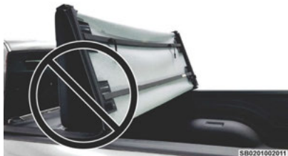
Incorrect Folding — Will Cause Damage
