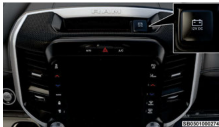
Power Outlet — Top Of Center Stack
