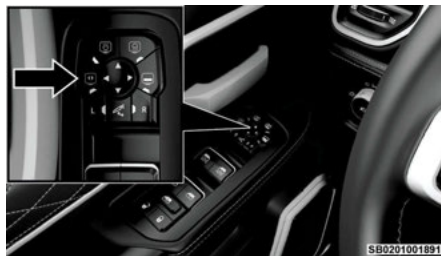
Forward and Reverse Light Switches
