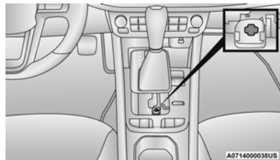
Gear Selector Override Access Hole
