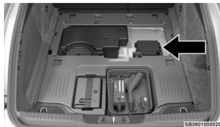
Rear Power Distribution Center
