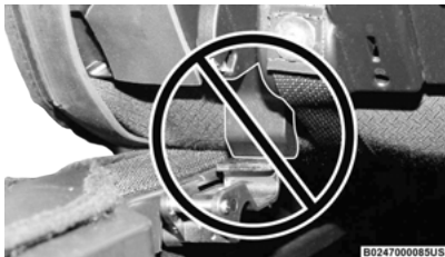
Incorrectly Seated Retainer
