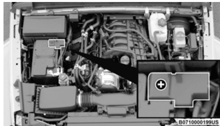
Positive (+) Battery Post – Gas Engine
