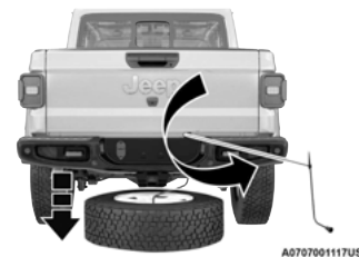
Pulling The Spare Tire Out
