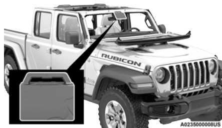
Protective Cover Installed
