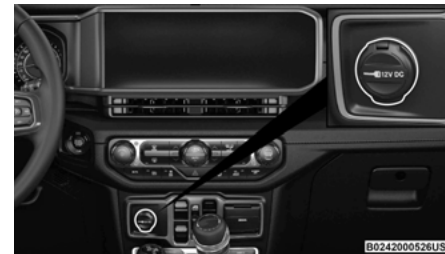
Front Power Outlet
