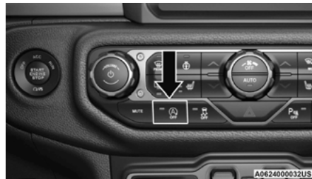
Stop/Start OFF Switch
