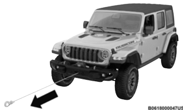
Pulling Synthetic Rope
