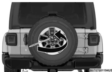
Removing The Spare Tire
