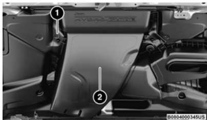
First Water Separation Chamber
