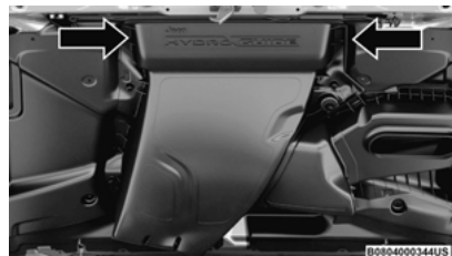
First Water Chamber Removal
