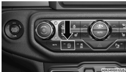
Stop/Start OFF Switch
