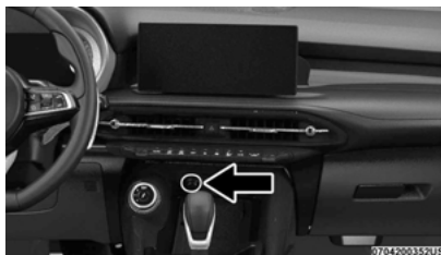
Power Outlet Location
