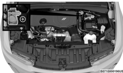
Positive (+) Battery Post
