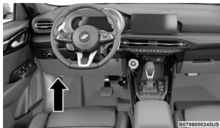
Interior Fuse Box Location
