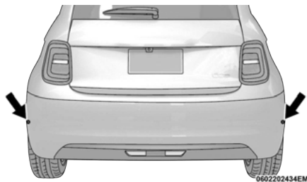
Radar Sensors Location
