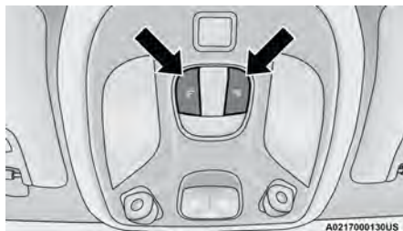
Overhead Light Switches
