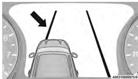
Lane Crossed (Flashing Yellow Line)
