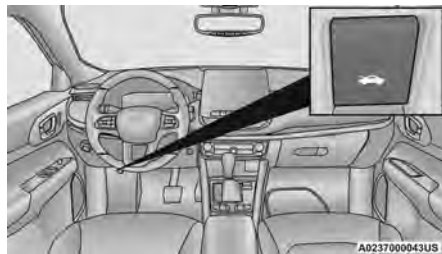
Hood Release Location (Underneath Instrument Panel)
