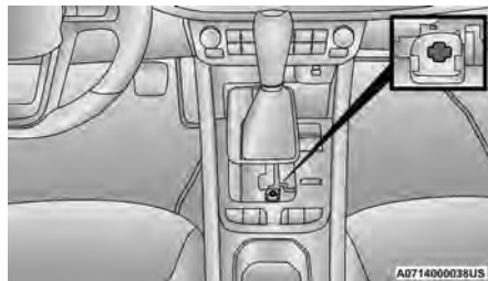
Gear Selector Override Access Hole
