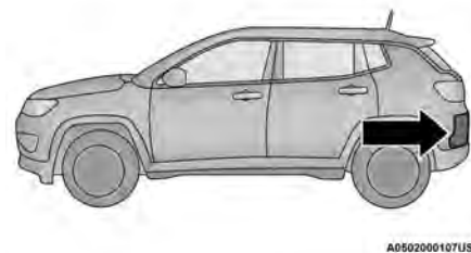
Radar Sensor Location (Driver Side Shown)
