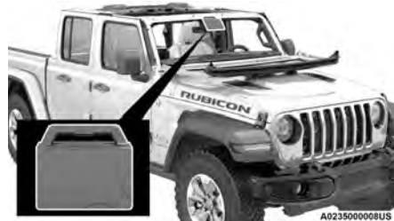
Protective Cover Installed
