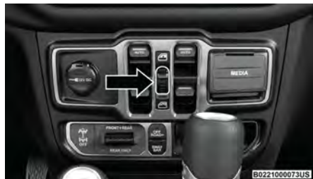
Window Lockout Switch
