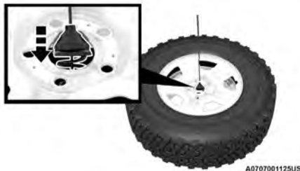
Reinstalling The Retainer
