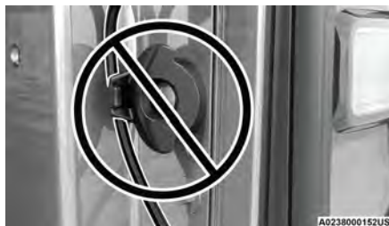
Incorrectly Seated Tailgate Strap
