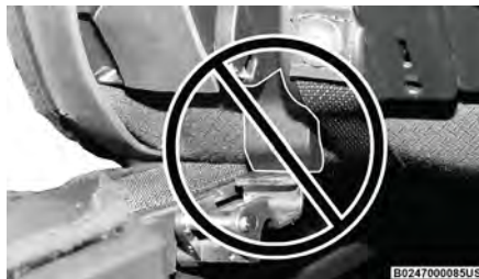
Incorrectly Seated Retainer
