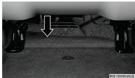
Rear Underside Of Front Seat Carpet Split
