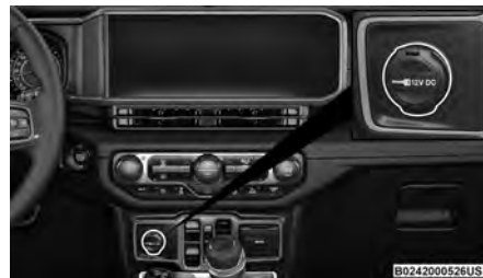
Front Power Outlet
