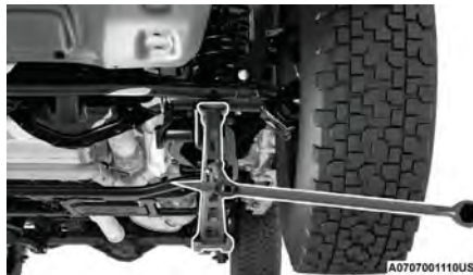
Front Jacking Location
