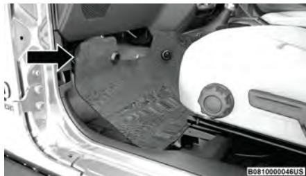
Front Carpet Pulled Away
