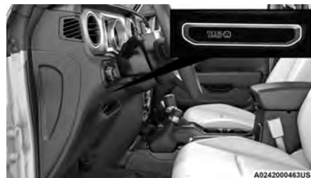
Power Inverter Switch (If Equipped)
