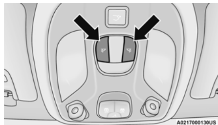
Overhead Light Switches
