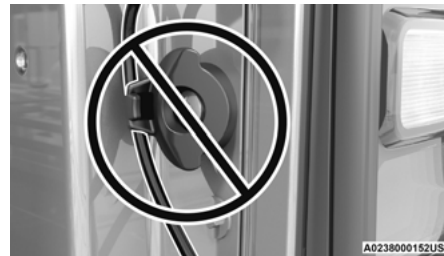
Incorrectly Seated Tailgate Strap
