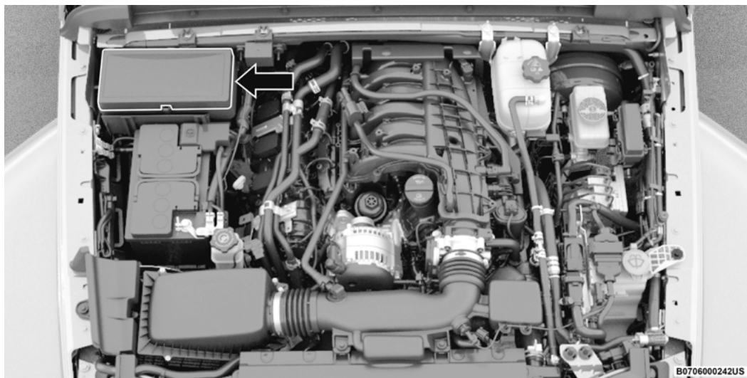
Power Distribution Center Location – Gas Engine
