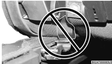
Incorrectly Seated Retainer
