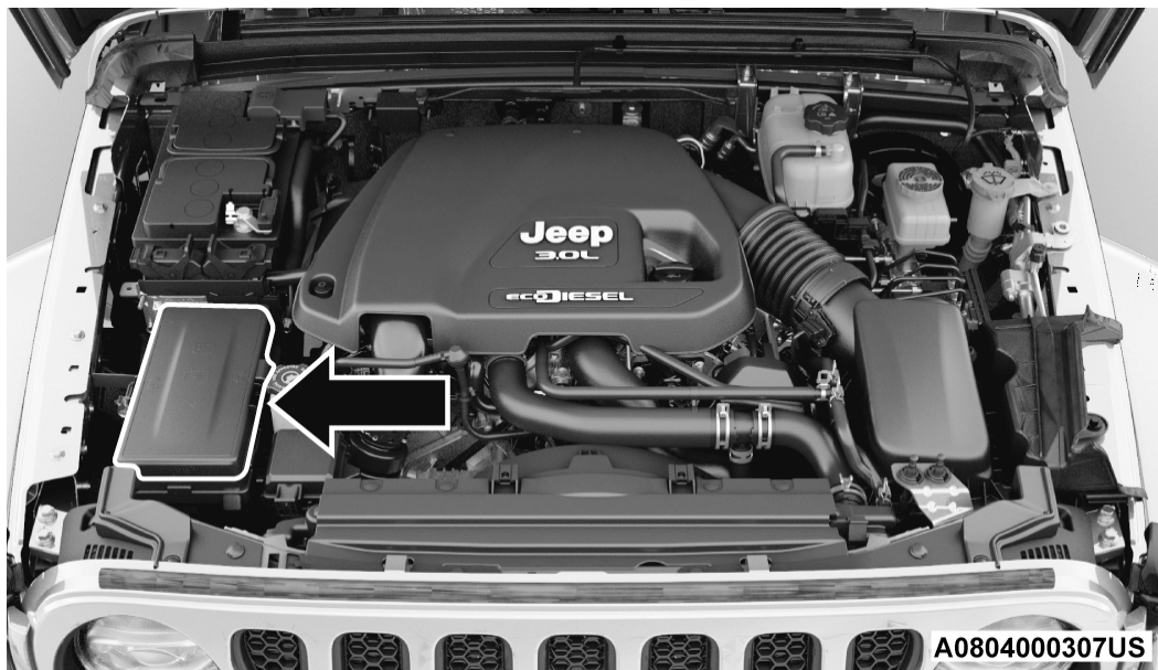
Power Distribution Center Location – Diesel Engine
