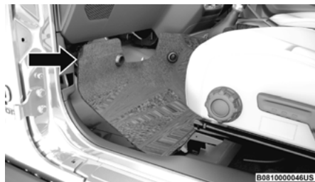
Front Carpet Pulled Away
