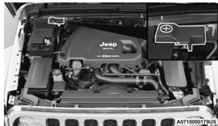
Positive (+) Battery Post – Diesel Engine
