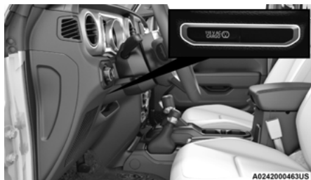
Power Inverter Switch (If Equipped)
