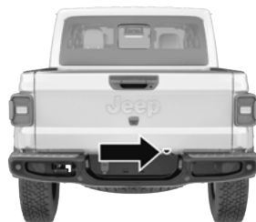
Access Hole Location
