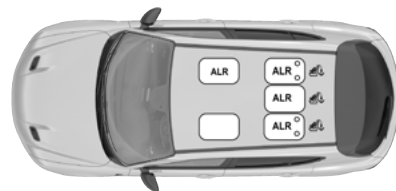
Switchable Automatic Locking Retractor (ALR) Locations
