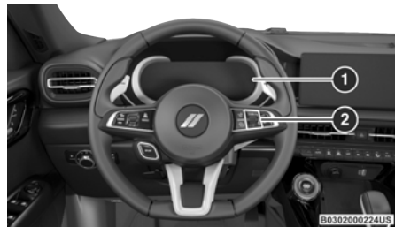
Instrument Cluster Display And Controls Location
