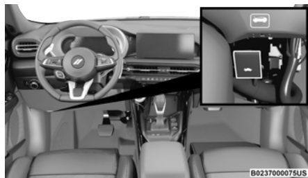
Hood Release Location (Underneath Instrument Panel)
