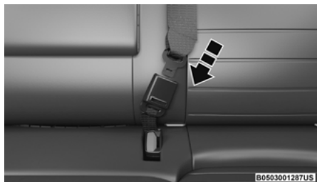
Inserting Mini-Latch Plate Into Mini-Buckle
