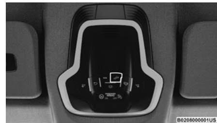
Volumetric/Anti-Lift Protection Button
