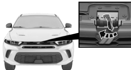
Hood Safety Latch Release Lever Location
