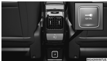
Rear Center Console Power Outlet — If Equipped
