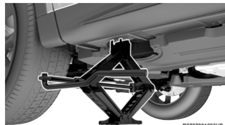
Front Jacking Location
