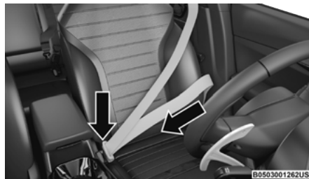
Inserting Latch Plate Into Buckle
