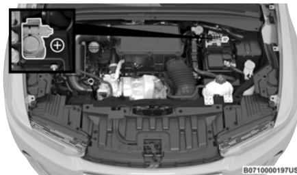
Positive (+) Battery Post
