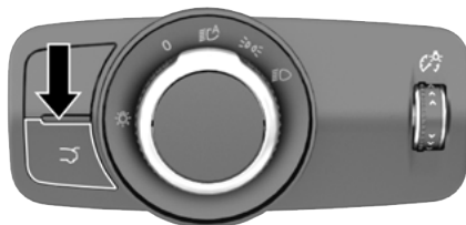
Headlight Switch Liftgate Button
