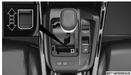
Gear Selector Override Access Location
