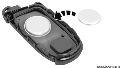
Key Fob Battery Replacement
