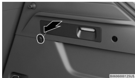
Fuel Door Emergency Release
