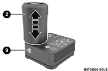
Sealant Cartridge Replacement
