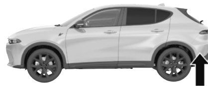
Radar Sensor Location (Driver Side Shown)
