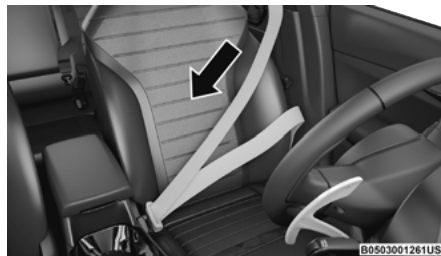
Pulling Out The Latch Plate
