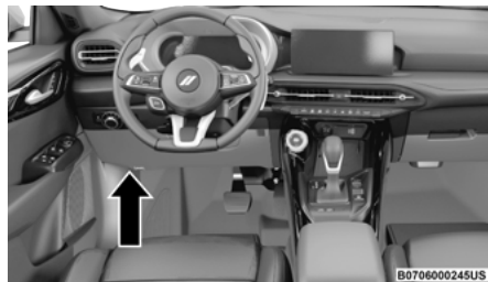
Interior Fuse Box Location
