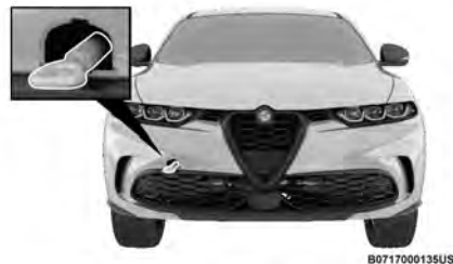
Front Tow Eye Installed
