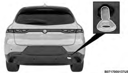
Rear Tow Eye Installed
