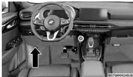
Interior Fuse Box Location
