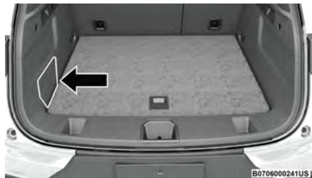
Rear Fuse Access Door Location
