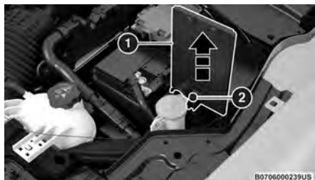
Fuse Box Cover And Locking Screw Removal
