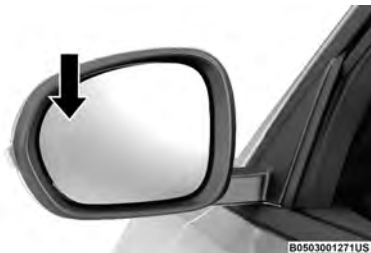
Warning Light Location
