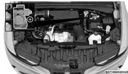
Positive (+) Battery Post
