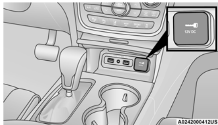
Front Power Outlet
