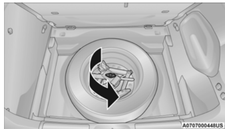
Removing Jack And Spare Tire Fastener
