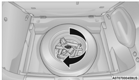
Reinstalling Jack and Tire Fastener
