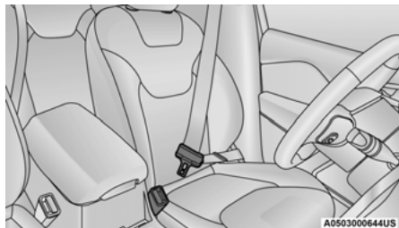
Pulling Out The Latch Plate
