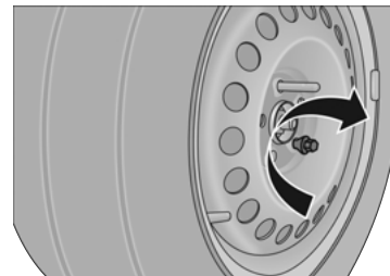
Installing Wheel Bolts
