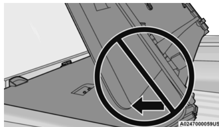
Incorrect Folding – Will Cause Damage
