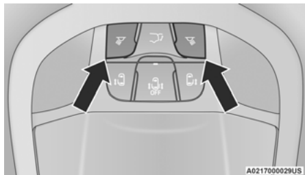
Courtesy Light Switches
