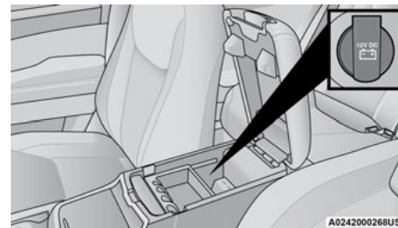
Center Console Power Outlet
