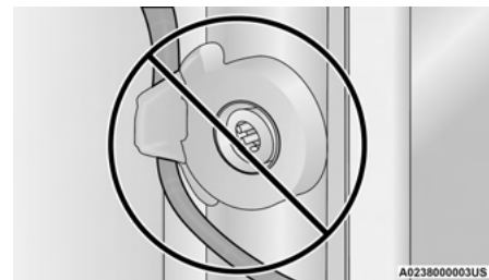
Incorrectly Seated Tailgate Strap
