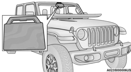
Protective Cover Installed
