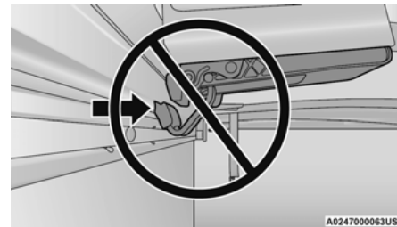
Improper Clamp Position
