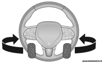
Remote Sound System Controls
