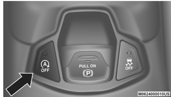
Stop/Start OFF Switch
