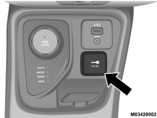
Front Power Outlet
