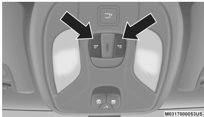
Overhead Light Switches
