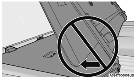
Incorrect Folding – Will Cause Damage
