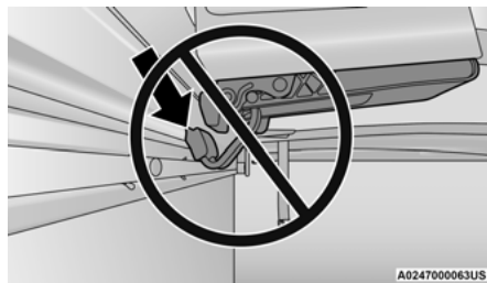
Improper Clamp Position
