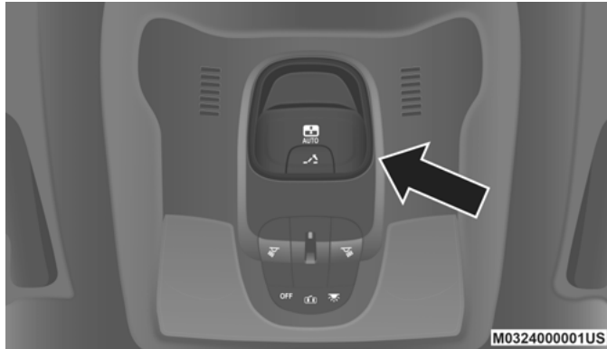
Front Panel Operation Switch
