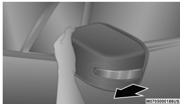
Removing the mirror cap
