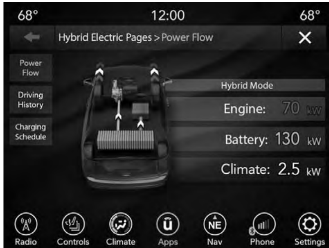
Power Flow Screen
