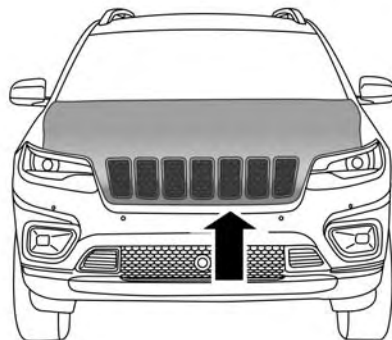
Hood Safety Latch Release Lever Location
