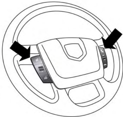
Remote Sound System Controls
