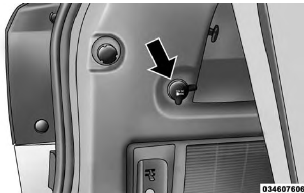
Rear Cargo Area Power Outlet
