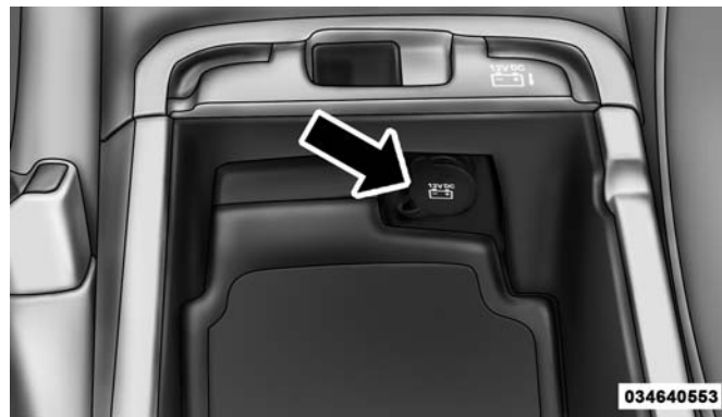
Front Center Console Outlet
