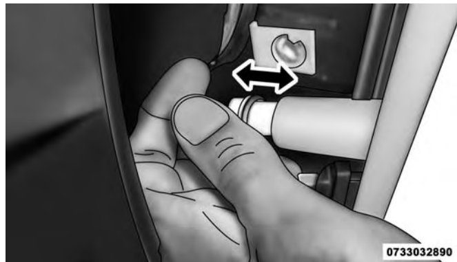
Front Side Marker Lamp Bulb Removal
