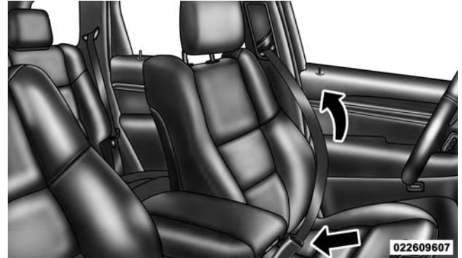
Positioning The Lap Belt
