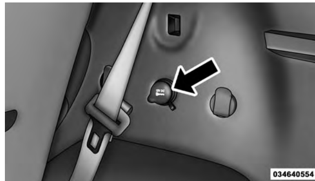
Rear Cargo Power Outlet
