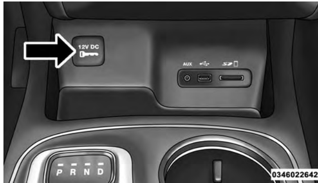
Front Power Outlet
