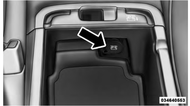
Front Center Console Outlet
