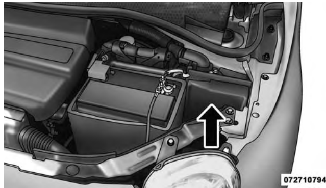
Front Distribution Unit
