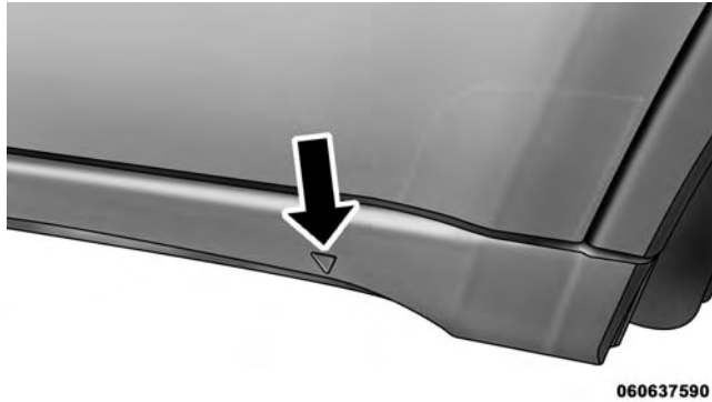
Lift Point On Sill Molding
