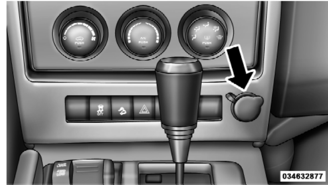
Front Power Outlet
