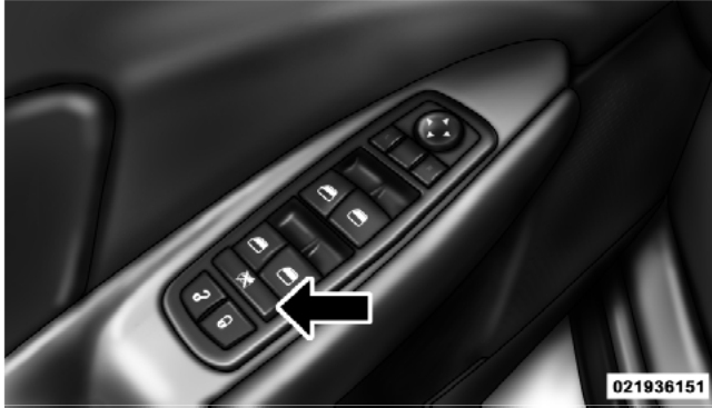
Window Lockout Switch
