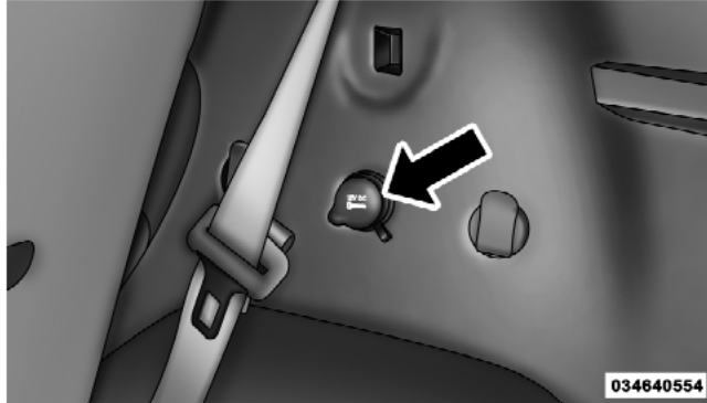
Rear Power Outlet
