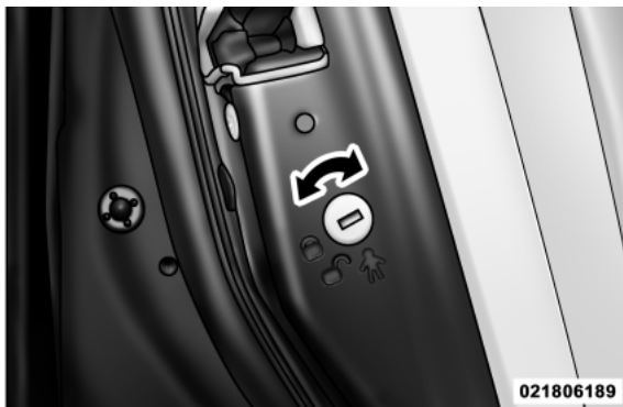
Child-Protection Door Lock Function
