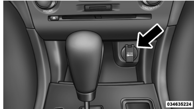
Front Power Outlet
